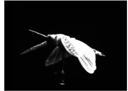
Locust in a wind-tunnel test, recorded using high-speed camera.
